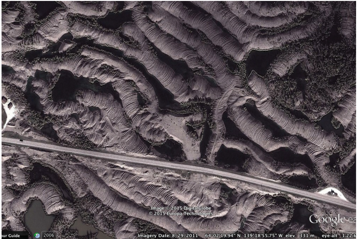
Above: Worm castings-like tailings. Note the vehicle on the far left side, on the highway, for scale. The pullout on the lower right side of the image includes the "Welcome to Dawson" sign.
